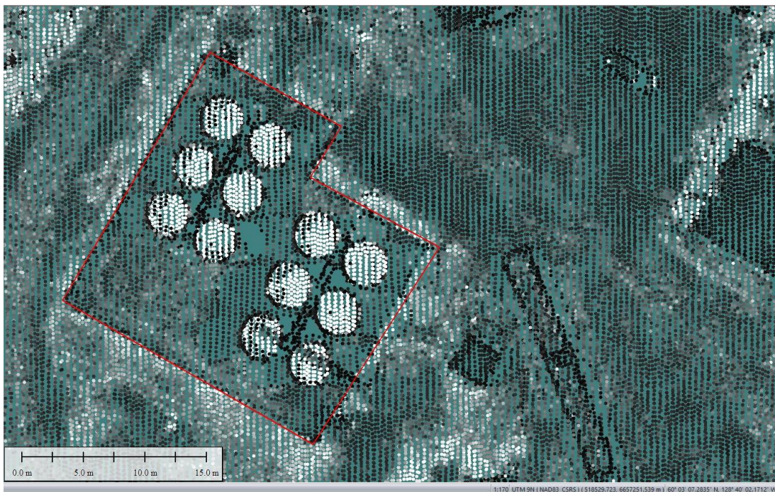
Figure 4 - Comparing LiDAR Horizontal Accuracy: Red lines are extracted from existing LiDAR data and overlaid on the current data.
