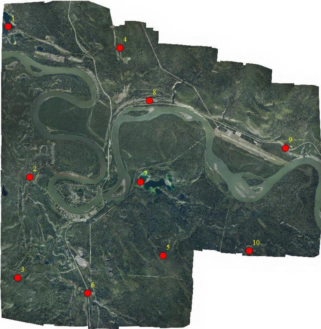
Figure 4- Location of orthophoto controls for LiDAR accuracy check
