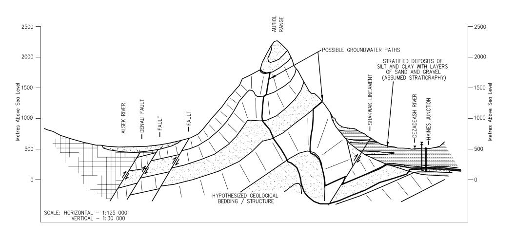
Figure 14, Pg. 62 Conceptual Hydrogeological Model of Well #5 Bedrock Structural Control
