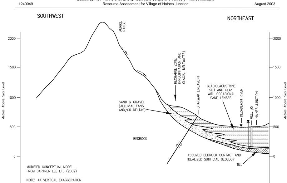
Figure 13, Pg. 60 Conceptual Hydrogeological Model of Well #5 Alluvial Fans/Deltas Control
